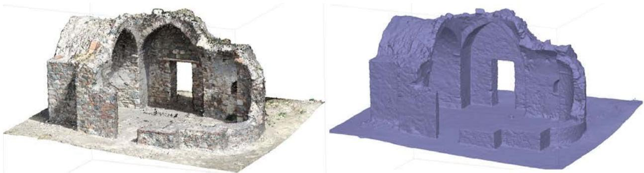
Figure 3: Left: Point cloud of church. Right: DSM of church
