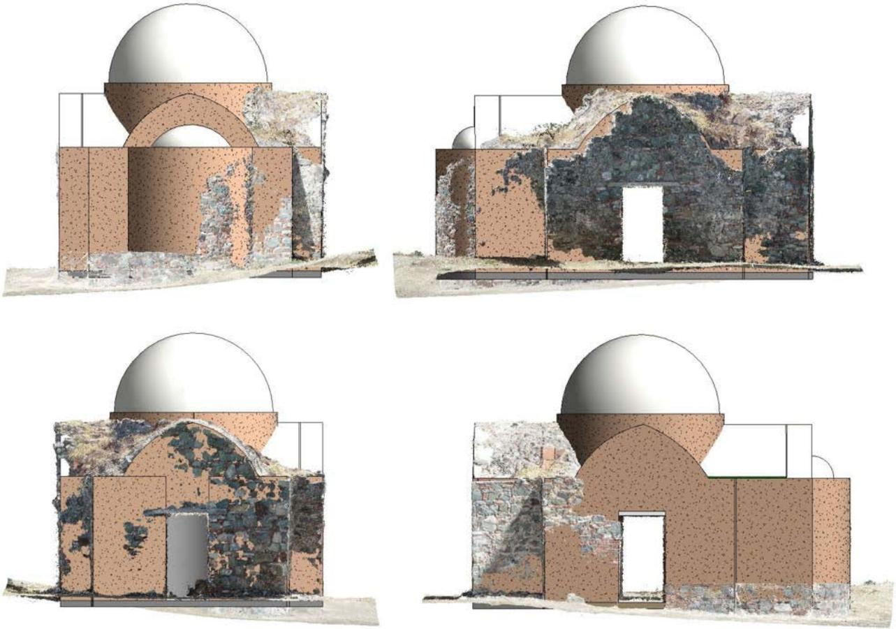
Figure 6: Elevations of reconstructed church from North, South, East and West with the original materials extracted from the digitized model
