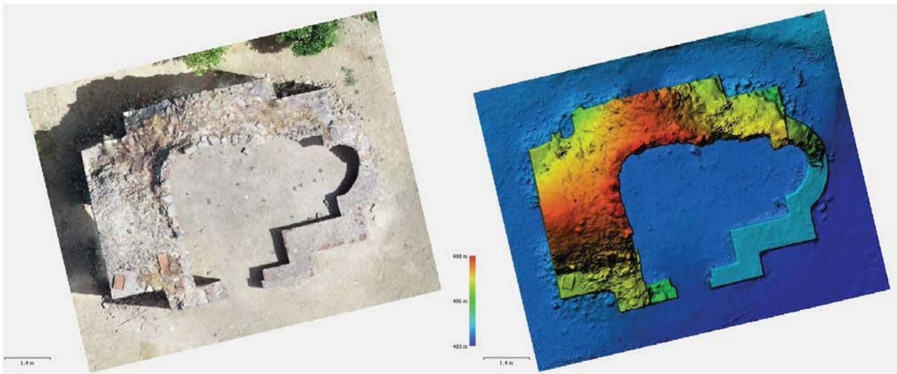
Figure 4: Left: Ortho-photo of the Church. Right: DEM of the Church
