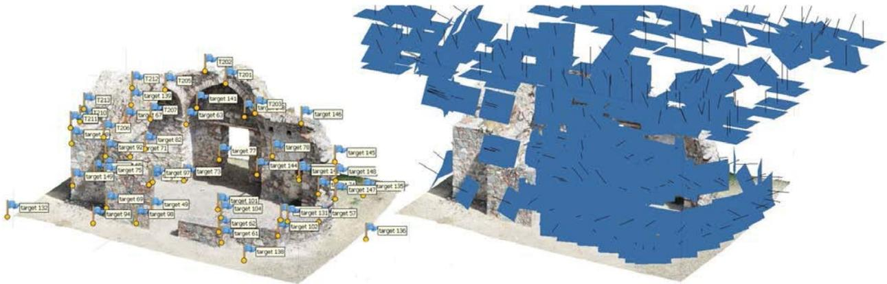
Figure 2: Left: Location of GCPs. Right: Image acquisition positions
