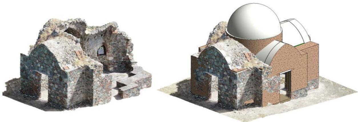
Figure 9: Left: 3D model of the existing Church; Right: 3D model of the reconstructed digitized model
